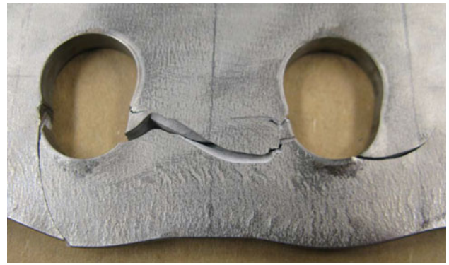
Fig. 10 Low-magnification micrograph showing overall morphology of failure of Plate #2
