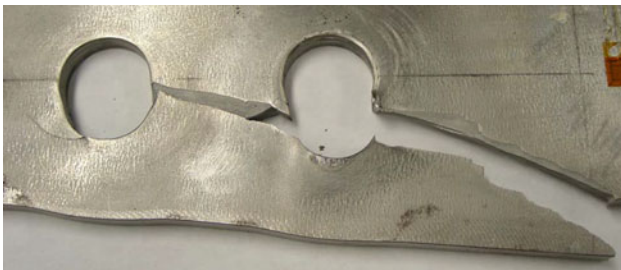
Fig. 9 Low-magnification micrograph showing overall morphology of failure of Plate #1
